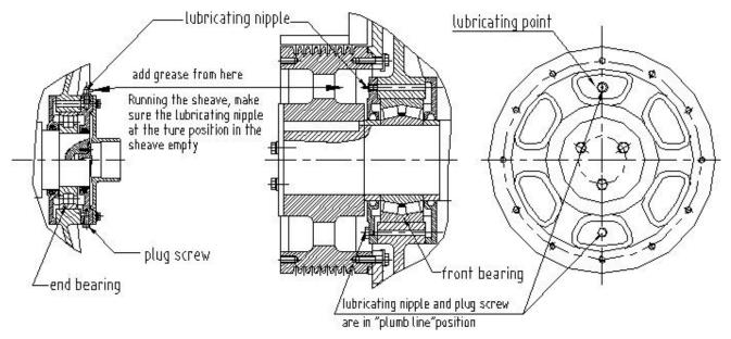
(2) Before doing this, remove the plug screw M10  $\times$  1 which protects the regreasing hole. Use 3# lithium (soap) grease. The refilled grease should exert only slight pressure on the grease column.
