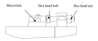
1) If it is the first time to adjust the micro switch, please rotate the hex head blot to the switch side, until it touch the contactor of micro switch.
